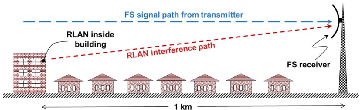
Figure 1: RLAN interference from inside building
